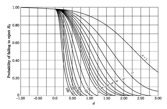
with  $d = (\mu_1 - \mu_2)/\sqrt{\sigma_1^2 + \sigma_2^2} = 10/\sqrt{128} = 10/(8\sqrt{2}) = 0.88$  (1/2 Mark) and  $\beta = 0.1$ . (1/2 Mark) This gives a minimum sample size of about  $n_1 = n_2 = 17$ . (2 Marks for any number greater than 15 and not greater than 20).
